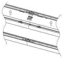
Seamless connection: Joint ceiling plate with connect accessory by screws, fix the fixture on the ceiling plate through connector.
