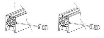
Fix the module into ceiling plate, make connector hook hang the ceiling plate.
