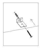
Knock the plastic anchors into the wall, fix the wall plate on the wall.
