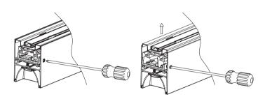
Press the connectors, take out the ceiling plate.
