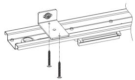
Fix the ceiling plate on the wall plate.
