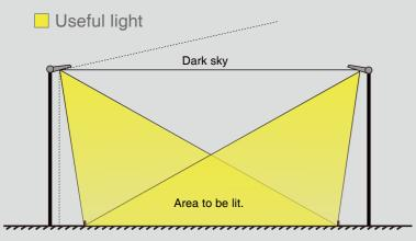
iBoard LED Floodlight is specially designed for sports fields, minimizing loss of light and light pollution.
